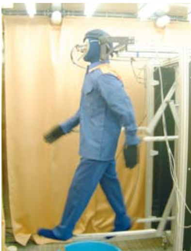
Analysis of thermal resistance of protective clothing using the sweating-walking thermal mannequin.
