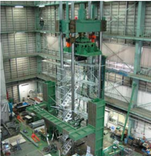
Performance test of temporary structures.
