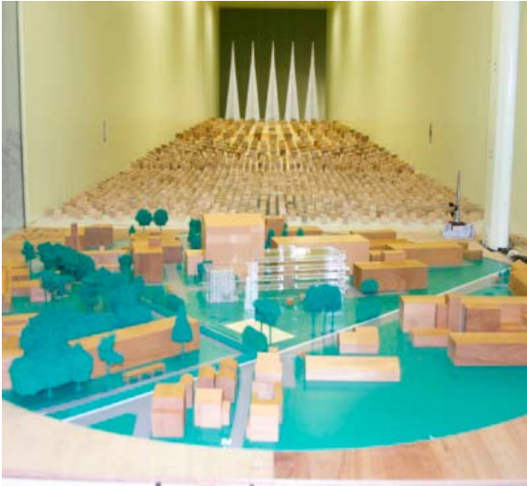
Wind tunnel tests for prevention of collapsing of temporary structures due to strong winds.
