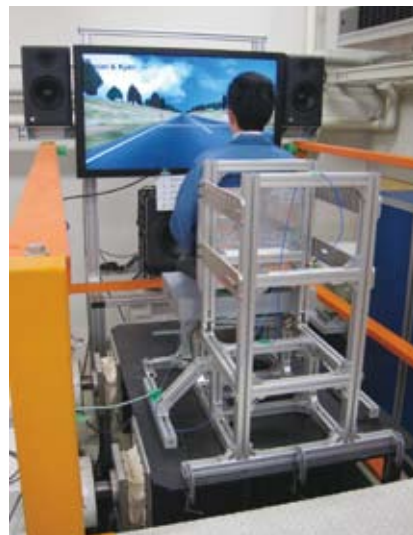
6DOF vibration test rig.
