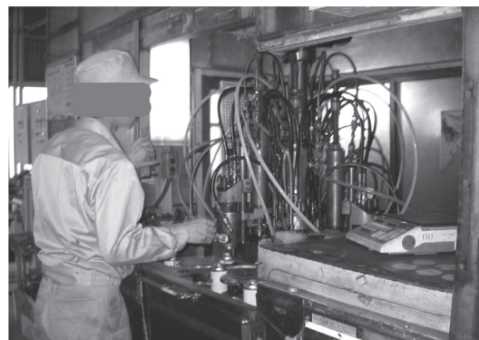
Fig. 6. Filling a canister with methyl bromide. The hood is lifted and the gas injector is adjusted manually.
