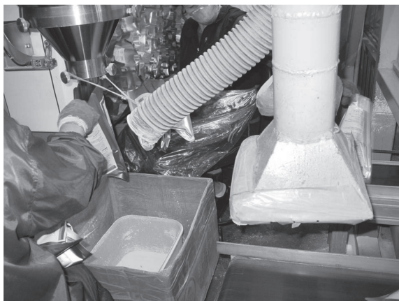
Fig. 1. A worker holds the bag under the hopper to fill with chlorpyrifos powder by hand.
