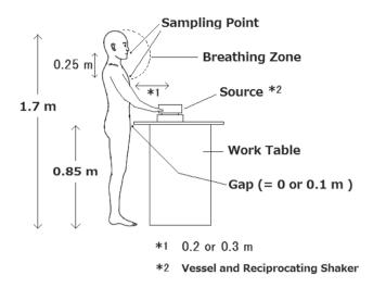
Fig. 1. Source location and sampling points in the experiment.
