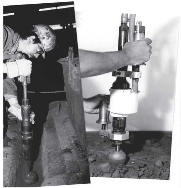
Fig. 3. A conventional rammer, and a prototype of low-vibration rammer 2 ).
