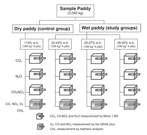
Fig. 3. Schematic of study samples in experimental pits and gas measurement
