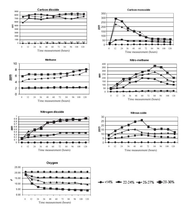
Fig. 4. The mean concentration of various gases over time at different moisture content of piled paddy
