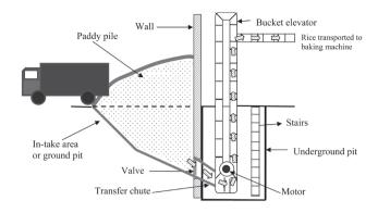
Fig. 1. Drawing of loading area and underground pit in rice mills
