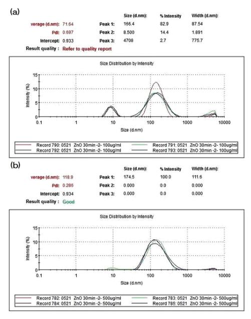
Fig. 2. Report of size distribution of ZnO nanoparticles suspensions dispersed by a probe-type sonicator at 20 W, 80% pulse mode, for 30 min, at measure concentrations of: (a) 100 and (b)  $500 \mu g/ml$ .
