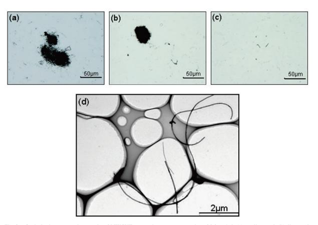
Fig. 8. Optical microscope micrographs of MWCNT suspensions at concentration of 2.0 mg/ml: (a) un-dispersed, (b) dispersed by a cup-type sonicator at 100 W, 80% pulse mode, for 10 min, and (c) for another 10 min; and (d) TEM micrograph of MWCNT sonicated twice.
