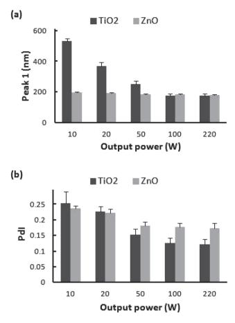
Fig. 7. Size characterization of  $TiO_2$  and ZnO nanoparticle suspensions at concentration of 0.5 mg/ml dispersed by a cup-type sonicator at 10, 20, 50, 100, or 220 W, 80% pulse mode, for 10 min: (a) peak 1 and (b) PdI. Data are mean  $\pm$  SD.
