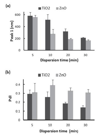
Fig. 3. Size characterization of  $TiO_2$  and ZnO nanoparticle suspensions at concentration of 0.5 mg/ml dispersed by a probe-type sonicator at 20 W, 80% pulse mode for, 5, 10, 20, or 30 min: (a) peak 1 and (b) PdI. Data are mean  $\pm$  SD.
