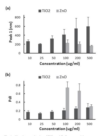
Fig. 1. Size characterization of  $TiO_2$  and ZnO nanoparticle suspensions at concentration of 0.5 mg/ml dispersed by a probe-type sonicator at 20 W, 80% pulse mode, for 30 min, being measured by DLS at concentrations of 10, 25, 50, 100, 200, and 500  $\mu$ g/ml: (a) peak 1 and (b) PdI. Data are mean ± SD.
