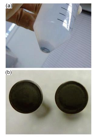
Fig. 6. (a) Black sediment at the bottom of a sample sonicated by a probe-type sonicator at 20 W, 80% pulse mode, for 30 min after 2 hours on standing and (b) the tip surface of unused probe (left) and abrased probe (right).
