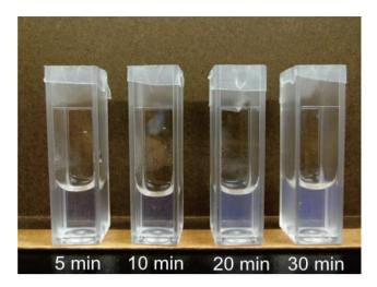
Fig. 5. Change in the turbidity of filtered  $TiO_2$  nanoparticle suspensions dispersed by a probe-type sonicator at 20 W, 80% pulse mode, for 5, 10, 20, or 30 min at concentration of 0.5 mg/ml.
