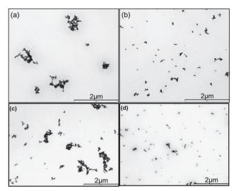
Fig. 4. TEM micrographs of  $TiO_2$  nanoparticle suspensions at concentration of 0.5 mg/ml dispersed by (A) a probe-type sonicator at 20 W, 80% pulse mode, for (a) 10 min and (b) 30 min; (B) a cup-type sonicator at (c) 50 W and (d) 100W, 80% pulse mode, for 10 min.
