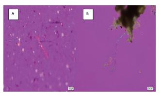
Fig. 2. (A) PLM micrograph of airborne chrysotile fibers in the asbestos cement sheet sample to site demolition; (B) PLM micrograph of airborne chrysotile fibers in the ventilation ducts and chimney pipes sample to the site.
