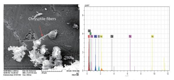
Fig. 4. SEM image and EDS spectrum from sample of asbestos cement sheet showing crysotile fibers (red arrows). Magnification, 2,000×.
