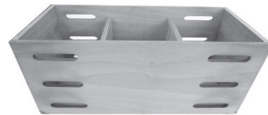
Fig. 1. Photograph of the experimental box with three different box handle positions (upper, middle, lower) on each side.
