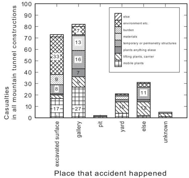
Fig. 4. Relationship between number of casualties and places where accidents happen with the causes which trigger the accidents in NATM and mountain tunneling methods.
