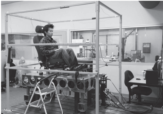
Fig. 1. A human vibration simulator was designed for this study. An actual vehicle's seat was mounted on a vibration table. Hydraulic actuator located at the corner of the table will provide multi-axial input to the volunteer. Volunteer was asked to take a seat and assume a comfortable position with their hands on the lap. Feet were placed on the footrest to isolate the vibration from the floor.
