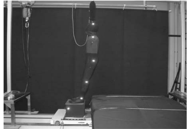
Fig. 1. The dummy suspended on the moving floor and the linear accelerator.
