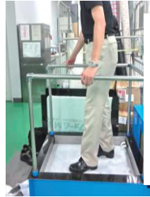
Figure 6. An example of the ice slip test device
