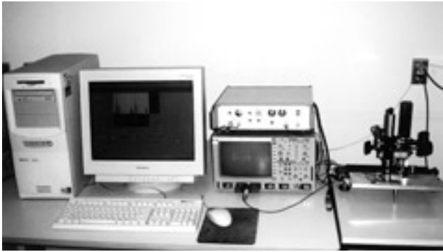
Photo 1 Photograph of the system developed to undertake ultrasonic measurement.
