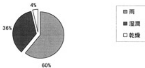
Fig. 17 Influence of wet condition in working area on electric shock. 感電した作業場所の環境条件
