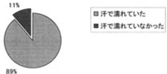
Fig. 19 Influence of wet condition of work clothes on electric shock. 感電時の作業着衣の状況
