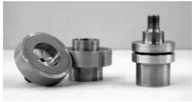
Photo. 2 Trial model of magnet loaded safety valve. 磁気式安全弁の構造
