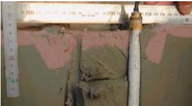
Photo. 1 State of soil around pile after experiment (Case 1) 実験後の杭周辺の地盤状態 (ケース 1)
