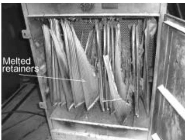
Fig. 1 A dust explosion in a bag-filter device during retrieving collected magnarium dust. マグナリウム粉じん回収中に爆発した集じん機
