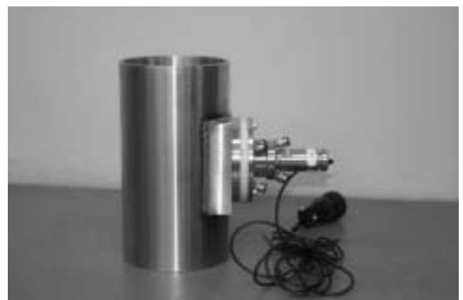
Photo. 3 Electrostatic field detector for pipe. 配管電界検出器
