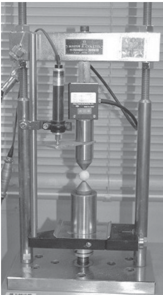
Fig. 4 Point load tests (left: apparatus for the point load test, middle: typical load - displacement relationship of point load test, right: illustrations of particles during test).
