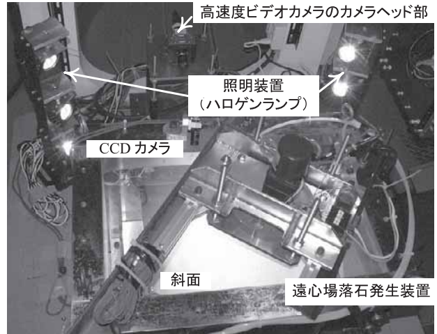
Photo 7 Closed-up view of the camera head and lighting system. カメラヘッドと照明装置の設置状況
