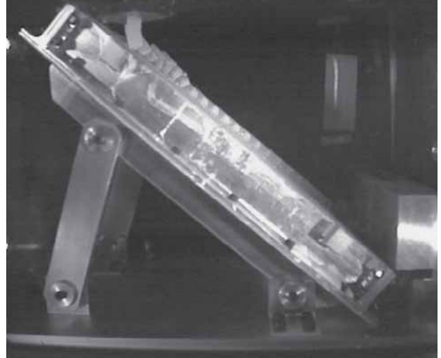
Photo 12 Simulated trajectory of falling mixture sphere while loading slide door of multiple ball-dropping system (RF-02-4). 混合試料躯体の落石模型による落石軌跡の一例
