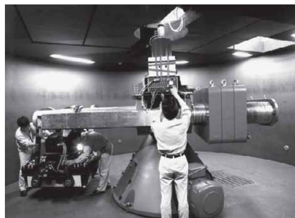
Photo 10 Centrifuge produced by Actidyn. (Nikken Sekkei Nakase Geotechnical Institute) Actidyn社の遠心模型実験装置 (日建設計中瀬土質研究所)
