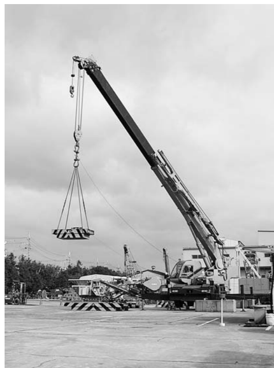
Fig.4 Stress measurement of the boom ブーム部応力の計測
