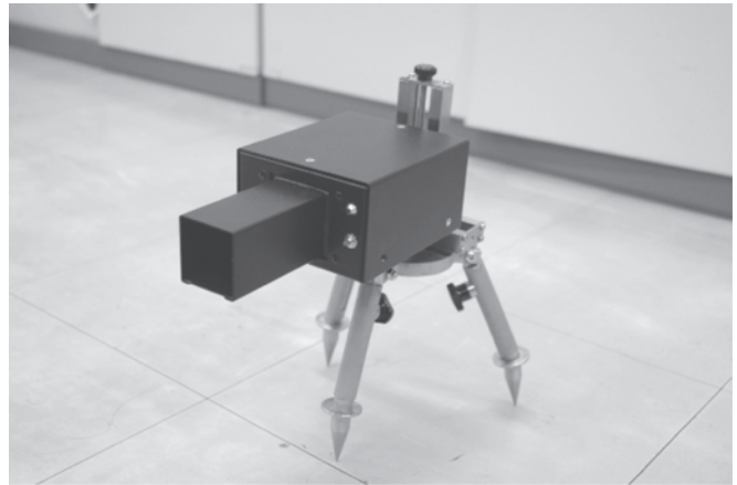
Fig. 25 Trial model of monitoring and alarm system for slope failure. 斜面崩壊警報システムの試作機
