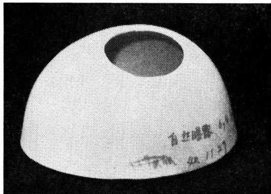
**Fig. 3** Six months exposed PE (3.6 kg)
